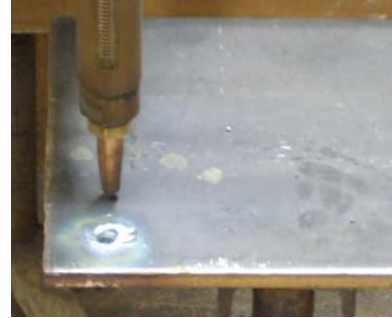
Fig. 14: Test specimen used in piercing tests.
