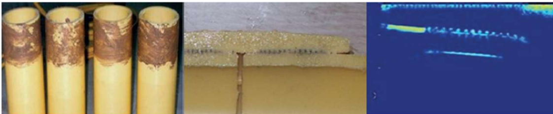
a) Pipes with soil contamination b) Cross-section of electrofusion socket joint c) related PAUT image
