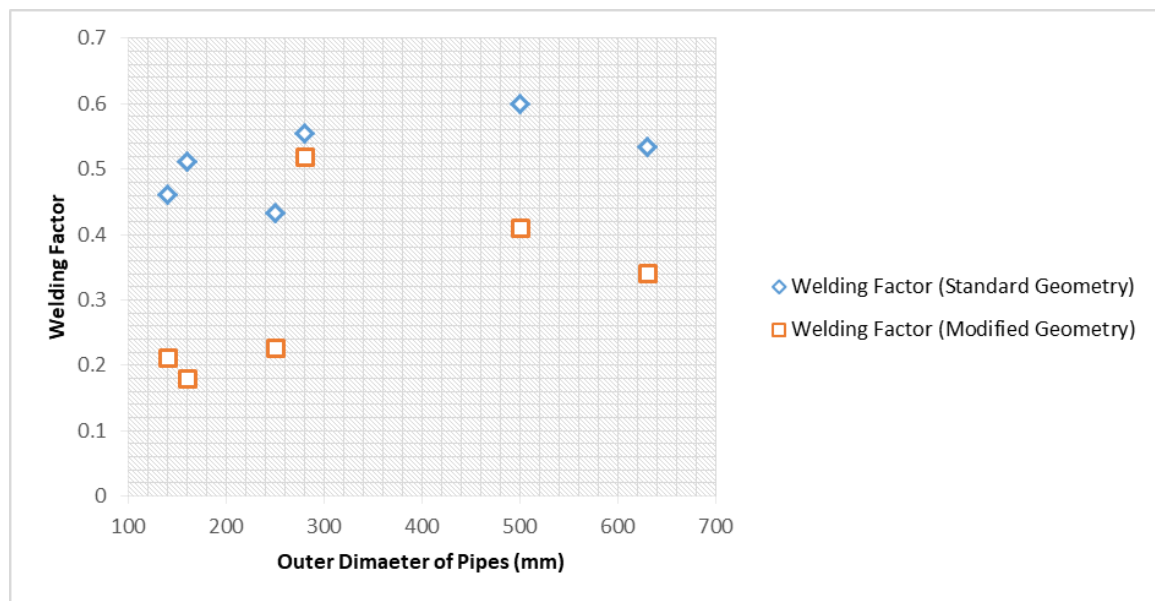
Figure 6-45, Welding factors for different pipe sizes
