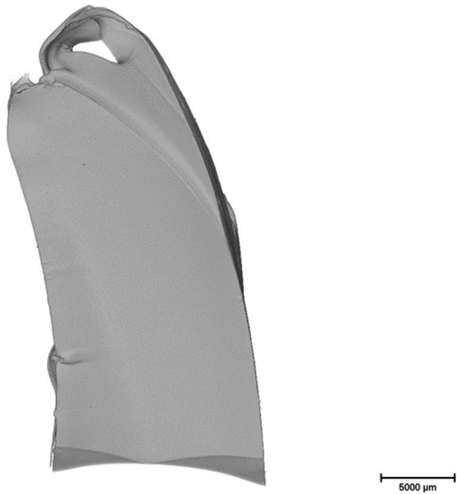
Figure 5-23, X-Ray photograph of ductile failure for specimen no 37
