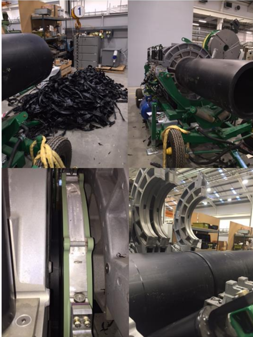
Figure 6-30, From top left clockwise, Trimming, pipe position in the machine, heater plate in place, final weld
