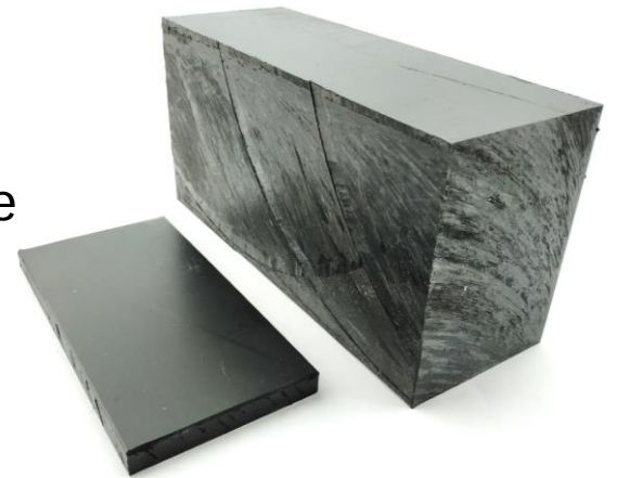
Comparison between usual laboratory dimensions (10 mm) and higher wall thicknesses (100 mm)
