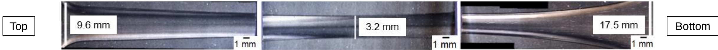
Microscopic image of PE100 RC, wall thickness 100 mm (polarised transmitted-light), welding parameters according to DVS
