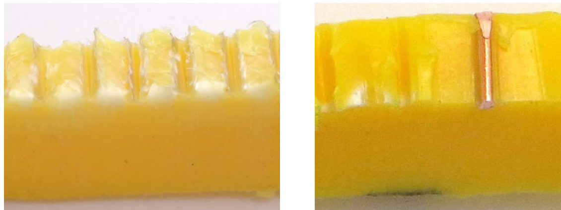
Figure 3: left: ductile area of the fracture surface after LSV testing, right: Brittle area of the fracture surface after LSV testing
