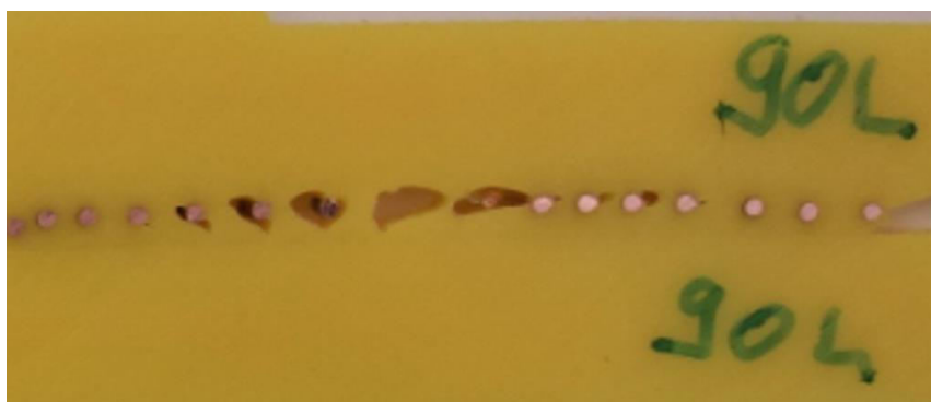
Figure 6: Formation of voids (fusion gap 0.80 mm, specimen with the highest number of voids).
