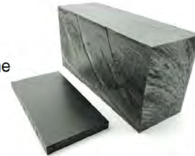
Comparison between usual laboratory dimensions (10 mm) and higher wall thicknesses (100 mm)
