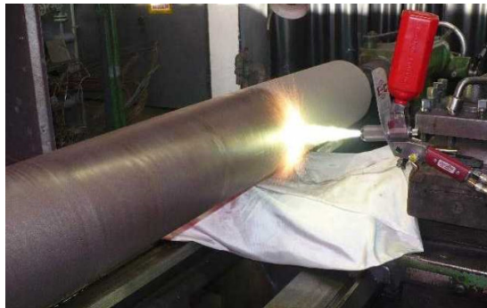
Spraying powders with CastoDyn DS 8000
