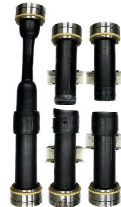
Figure A.6. Force-displacement results and corresponding photos of electro-fusion joints (normal, particulate contaminants, cold fusion) from the HAT test.
