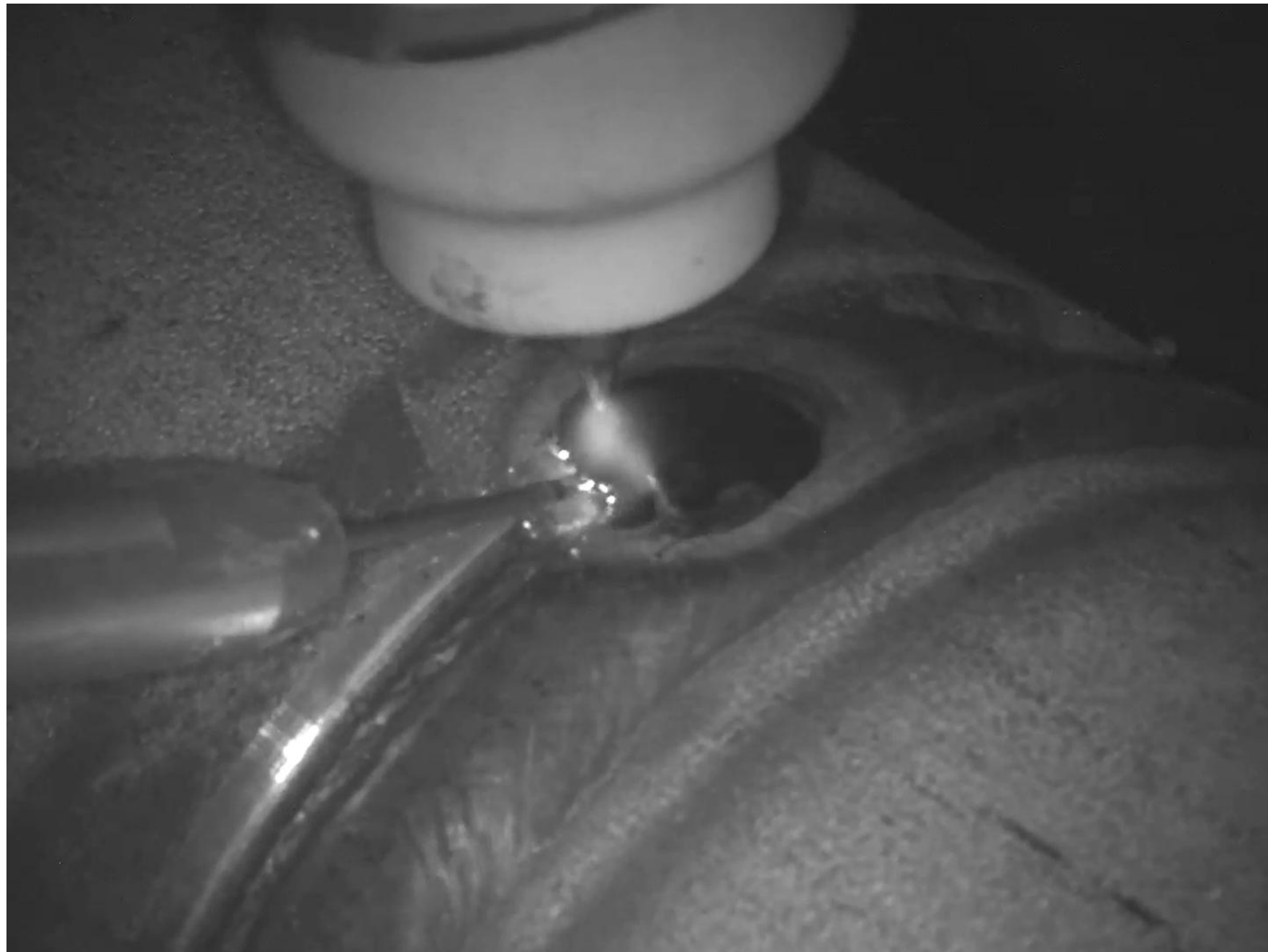
Video: Spatter caused by wire dragging
