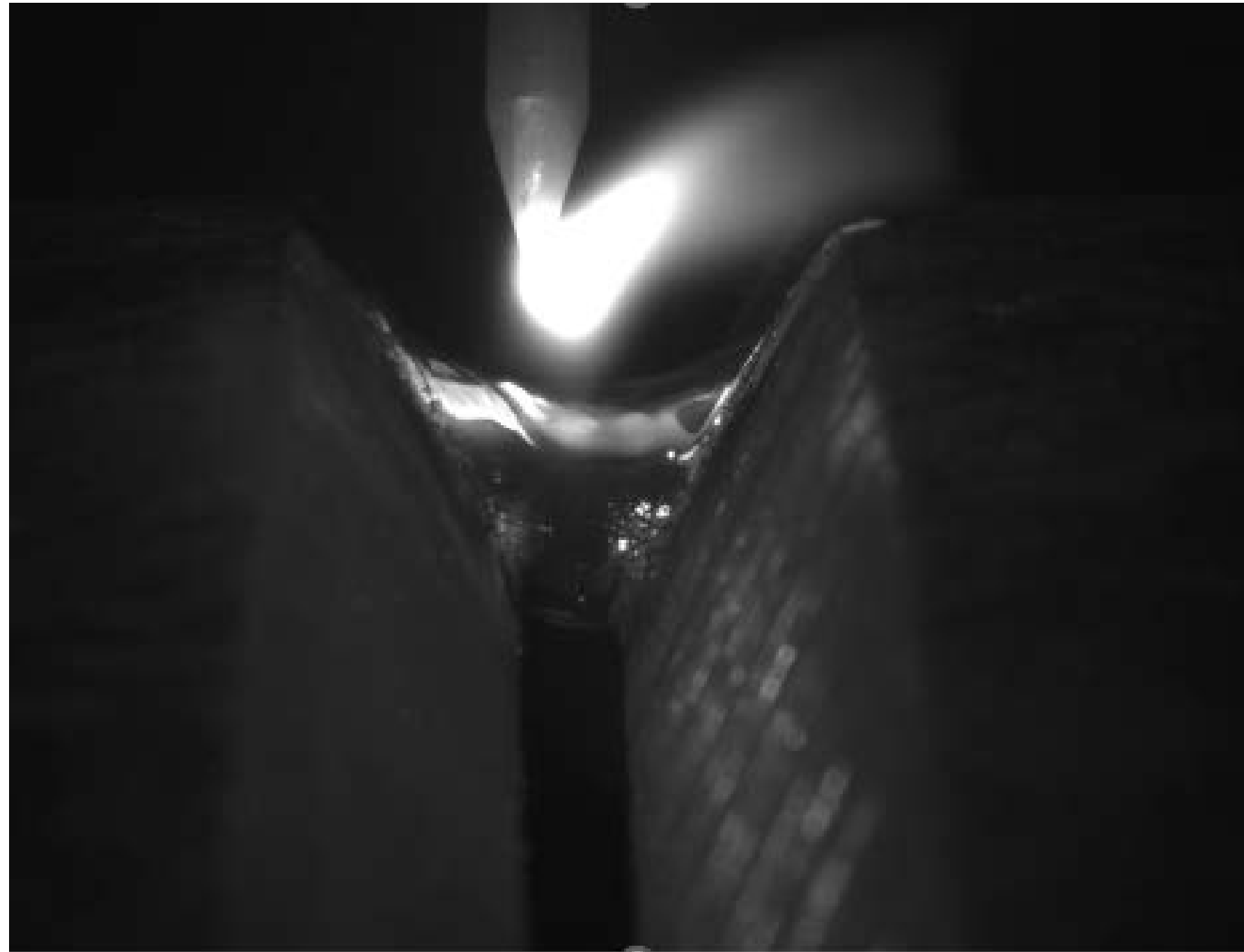
Video: Magnetic Arc Blow in TIG welding
