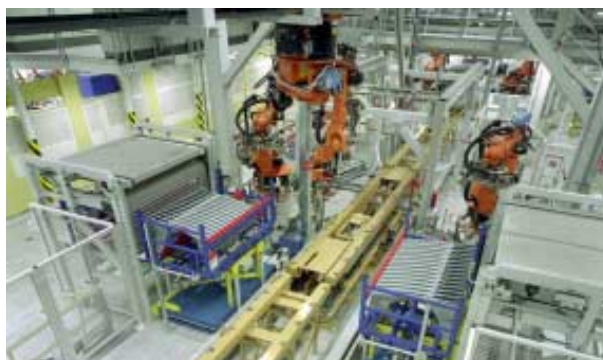
Figure 18. Flexible fender assembly station.
