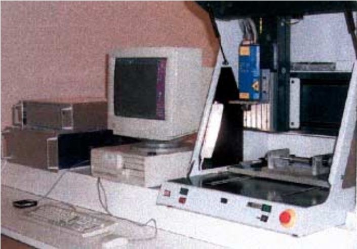
5. Compact welding plant with FLS iron and xyz-shift unit.
