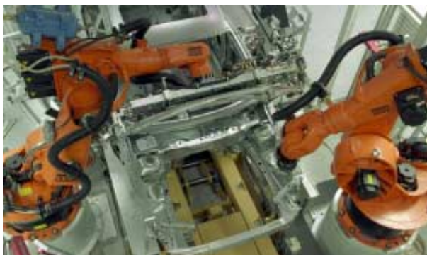
Figure 17. Flexible hood assembly station.
