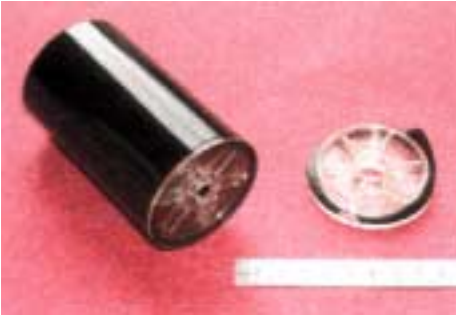
3. PA can: compression strength to 59bar.
