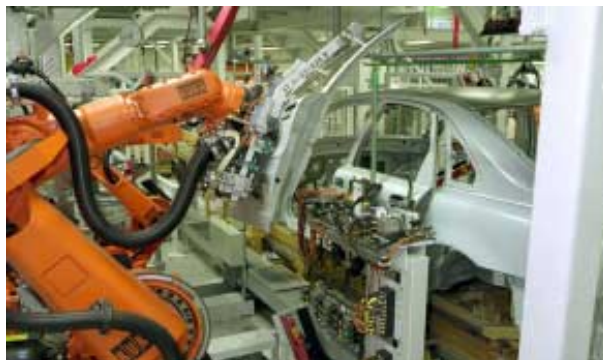
Figure 16. Flexible door assembly station.
