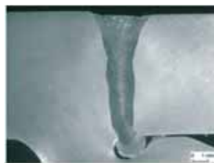
Laser MIG hybrid welding EN-AW 6005, t = 8 mm filler wire AlSi5 P_L = 10.5 kW v_w = 8 m/min
