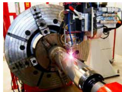
Fig. 4. Laser cladding hos Trio OilTec Services
