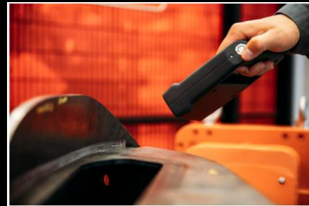
Handheld weld quality scanner - Wintoria FLEX
